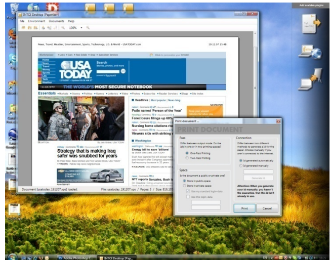
Figure 11: Our application can print an XPS document which automatically generates the Anoto pattern embedded in the printout. Moreover, the according page will be stored on the server.
